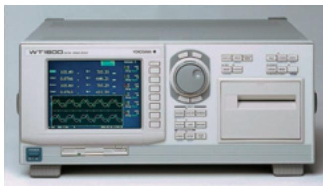
Measurements of powers (P, Q, S, D) and other data or electrical values (U, I,  $\varphi$ ,  $\lambda$ , etc.) can be easily distorted with complex signals. Numerous characteristics: permissible peak factor for an rms measurement, frequency pass band, sampling period, synchronisation (internal clock), update between two displays, must be known and controlled before taking measurements, which are quickly likely to be risky. Only suitable wattmeters or power analysers can provide this control.
