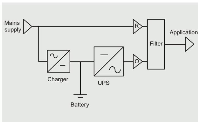
This technology is used for low powers that do not exceed a few kVA. The load (application) is supplied directly by the network via a simple filter that attenuates the disturbance.
