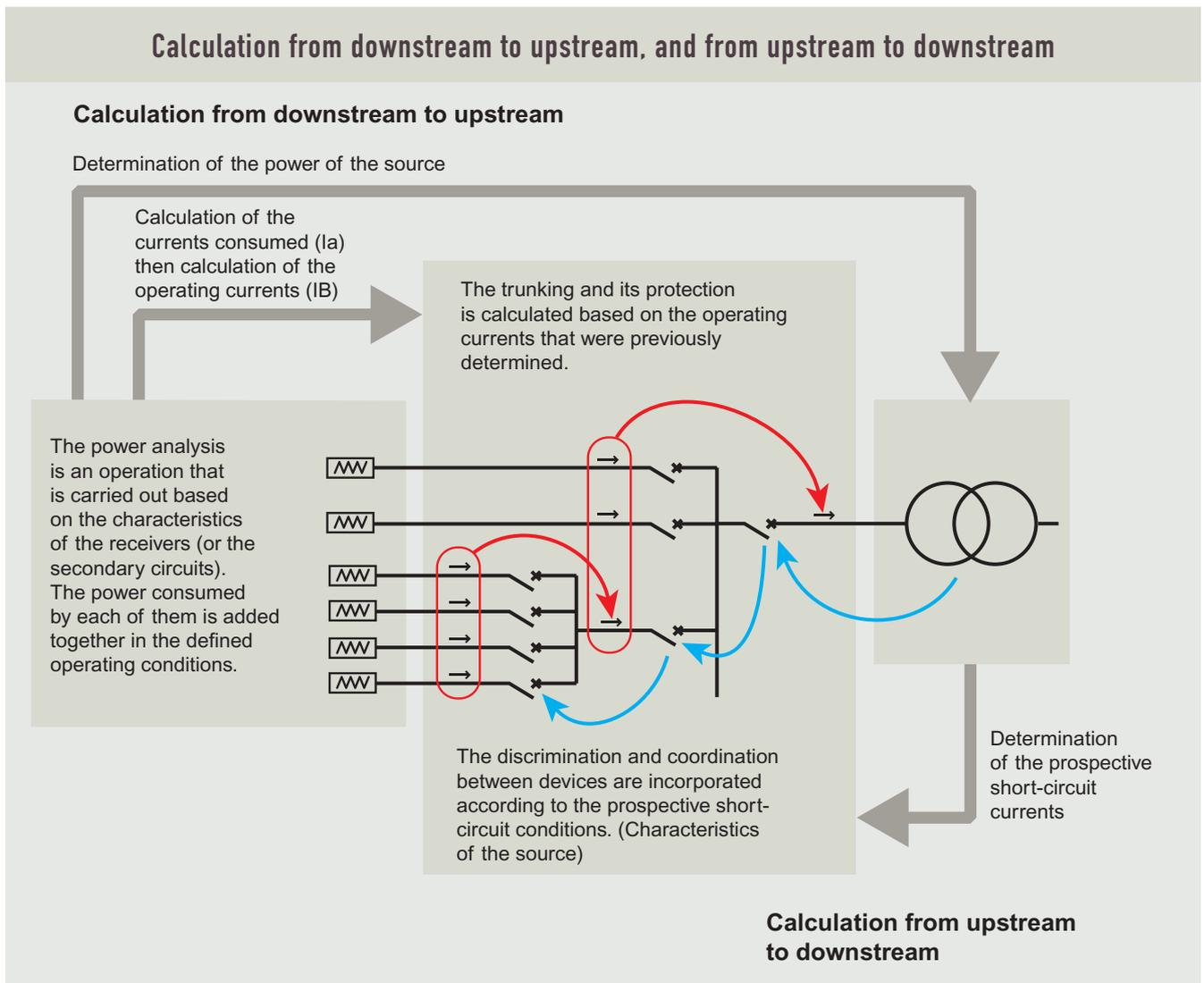
ANALYSIS OF THE LOADS, CALCULATION OF THE CURRENTS, POWER OF THE SOURCE
