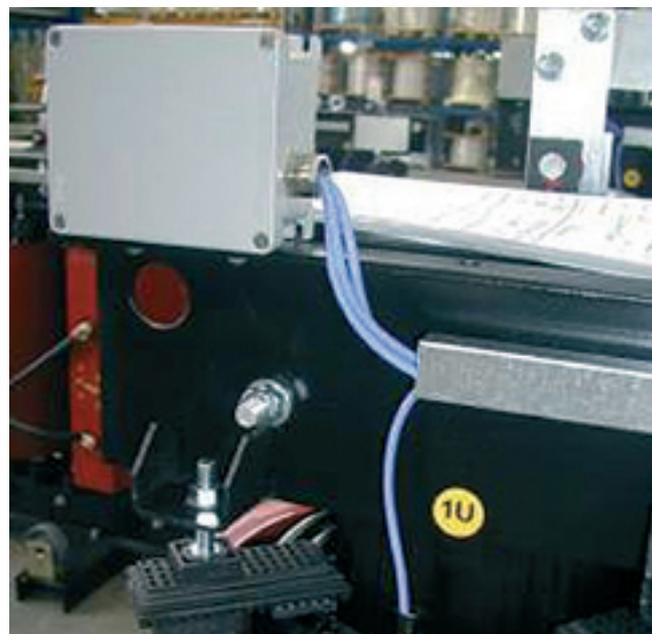
^ Example of installation of a Pt100 temperature control unit
