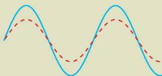
Example 1: Current and voltage in phase and sinusoidal
