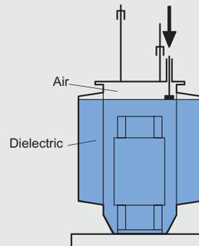
A quantity of air enters the surface of the oil and the cover allows the liquid to expand with no risk of overflowing. The transformer “breathes”, but the humidity of the air mixes with the oil and the dielectric strength deteriorates.
