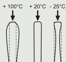
The overpressure due to the expansion of the liquid is absorbed by the folds of the tank.
