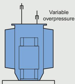
The tank is completely filled with liquid dielectric and hermetically sealed. There is no risk of oxidation of the oil.
