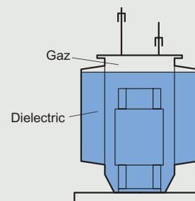
The tank is sealed and a cushion of neutral gas compensates for the variation in volume of the dielectric (risk of leak).
