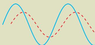
Example 2: Current and voltage sinusoidal but out of phase
