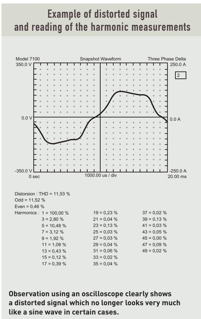
Most loads connected to the network are symmetrical (the current half-waves are equal and opposite). The total even-order harmonic distortion is generally zero. Three-phase, balanced, symmetrical, non-linear loads, with no connection to the neutral do not generate any 3rd order harmonics, or any harmonic orders that are multiples of 3. These cancel each other out in the triangular load circuit.
