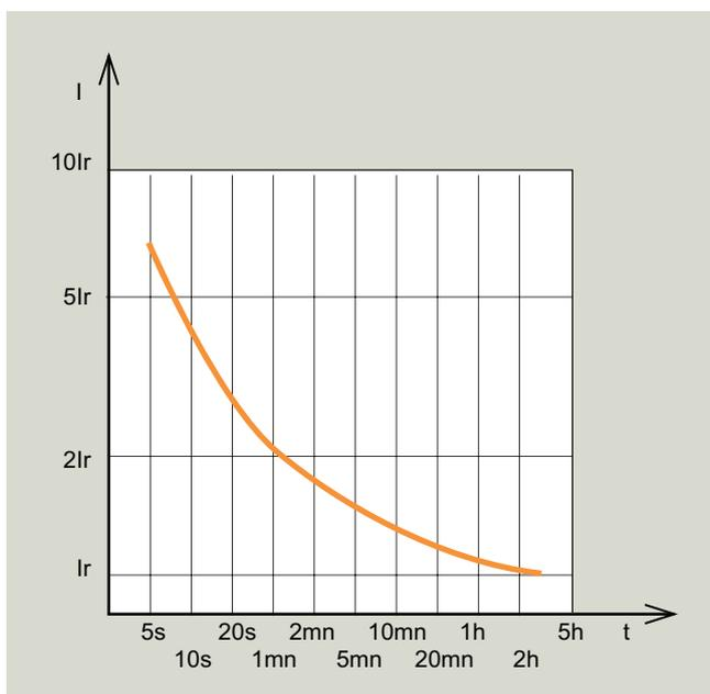
Overload capacity of an oil transformer
