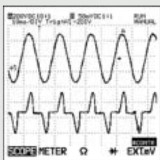
The voltage and the current are in phase but the current is not sinusoidal. The  $\cos \varphi$  has no significance. The actual power factor is less than 1. Distorting power is consumed.
