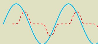
Example 4: Current and voltage out of phase and current non-sinusoidal
