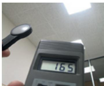
throughout the whole measurement period) must also be measured. The specific energy consumptions can be ascertained by multiplying the power by the recorded durations.
