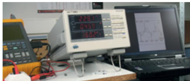
This device is used for measuring power. Current digital models can be used to access all values: P, Q, S, U; I,  $\cos \varphi$ , PF (power factor), etc., and even harmonic and frequency values. Some even carry out direct energy calculations by integrating the measurement time. These are referred to as power analysers.
