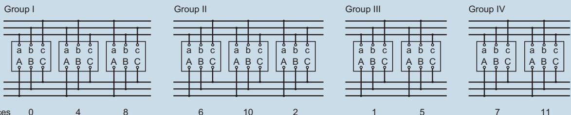
Parallel operation of transformers from different groups is possible by modifying connections, but they must be submitted for the approval of the manufacturer.
