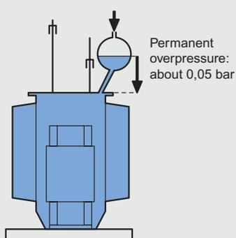
To limit the previous disadvantages, an expansion tank limits the air/oil contact and absorbs the overpressure. However the dielectric continues to oxidise and take in water. The addition of a desiccant breather limits this phenomenon but requires regular maintenance.
