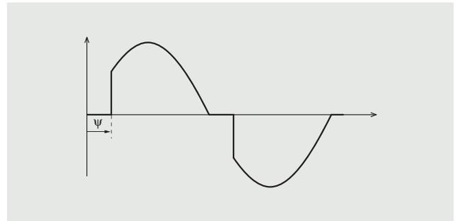
In the expression  $S = \sqrt{P^2 + Q^2 + D^2}$  the distorting power  $D$  is not zero and can be calculated, in the same way as  $P$  and  $Q$ , as a function of the non-conduction angle  $\Psi$ : the rms voltage and current, in the load, are expressed as a function of the same angle.
