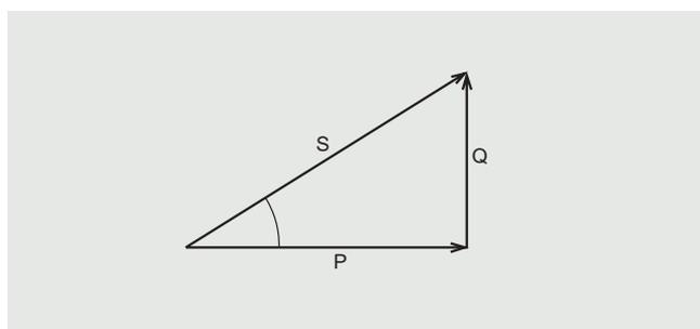
The active power  $P$  and reactive power  $Q$  are added together.
