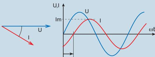
If these values are sinusoidal time functions, the current value can then be written in the form  $I = I_m \sin(\omega t + \varphi)$ .
