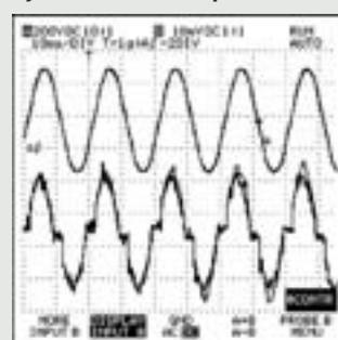
The power factor is improved by compensating for the distorting power (see below).
