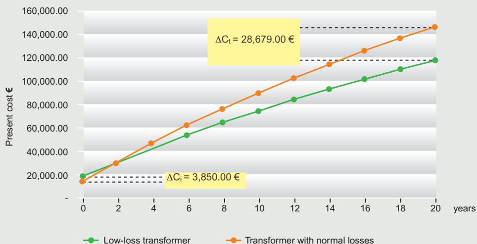
The final result is that transformer A is already cheaper after only two years. The  $\Delta$  initial cost of 3,850 Euros has been completely recovered and at the end of the transformer lifetime there is a saving of more than 28,000 Euros. To conclude, the initial cost does not represent a good parameter for the choice of
