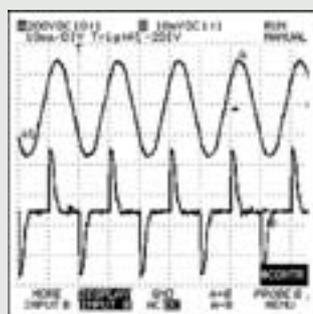
The current is ahead of the voltage and the load is distorted. Here too, the  $\cos \varphi$  has no significance. The power factor is less than 1 and must take account of the reactive power (due to the phase shift) and the distorting power.
