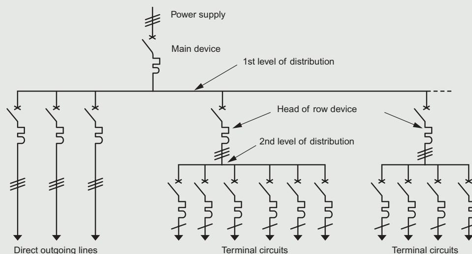
In most secondary or terminal distribution panels (see generic diagram on page 3), it is necessary to distribute three-phase and single-phase circuits. Some can supply receivers directly (direct outgoing lines) or supply points of use or small modular consumer units. In this case, it is not possible to keep to a single rule to determine the coincidence factors.
