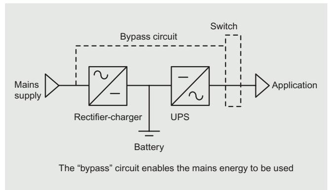
The most widely used technology for powers above 3 kVA, this is considered to provide the best performance. The load (application) is constantly supplied by the UPS, which ensures continuous regulation of the output voltage and frequency of the device ( $\pm 1$  to 3%). If there is a fault in the mains supply upstream, the load continues to be supplied with no switching.
