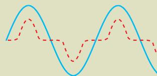
Example 3: Current and voltage in phase but current non-sinusoidal
