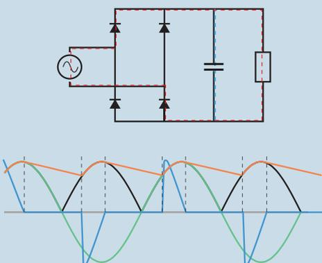
The principle is to rectify the mains supply, filter it and then install a switching device downstream that behaves like a resistive load. The disadvantage of the device is that it consumes a very distorted current (shown in blue): when the rectified mains supply (shown in black) exceeds the voltage of the filter capacitor (shown in orange), there is a sudden current surge.
